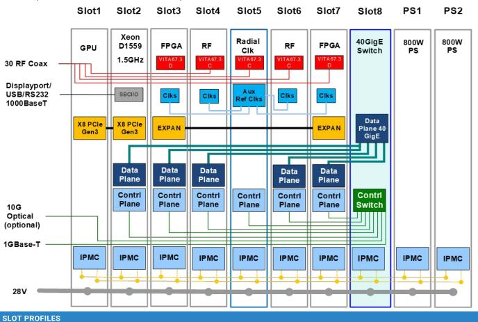
This 800 Series CMOSS SOSA System backplane support these slot profiles in alignment with the SOSA technical standard.
